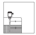
The product is the dielectricum. Due to the higher dielectric constant(DK-value) of the product against air, the capacitance value increases with the height of covering.
